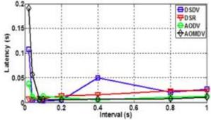
Figure 3. Packet interval vs. latency for 25 grid connected nodes
